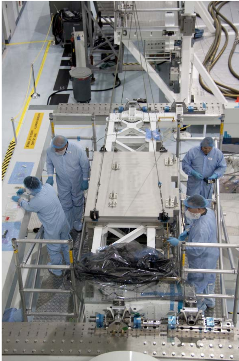
The top of the LMC is shown here with the special adapter plate installed to accommodate the Pump Module Assembly.
